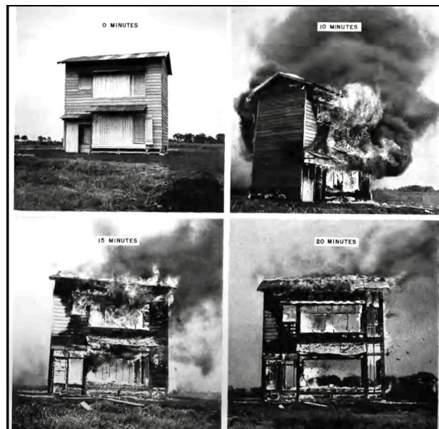
National Defense Research Council report showing stages of a Japanese house burning after 10, 15 and 20 minutes.
